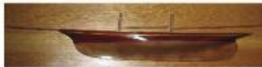
The "Livonia", LOA 127'0", Displacement 289 tons, Sail area 18,152 sq. ft., Designer and builder Michael Reaney.
